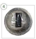
PACK & FILL DRUM Batteries/devices should be completely surrounded. Place the any remaining CellBlock into drum. Do not over fill. Any remaining can be used later.
