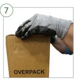
PLACE DRUM IN Place sealed drum back into overpack box. Use packaging tape to close the box and apply special permit and labels on the box.
