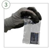
PROTECT BATTERIES Place each affected battery/ device into a bag and seal. 1 battery/device per bag.
