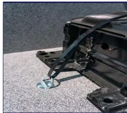
Secure battery inside crate in manner that prevents shifting in transport with non-conductive material. (Ex. Foam blocking, canvas strapping or bolting directly to crate.)
