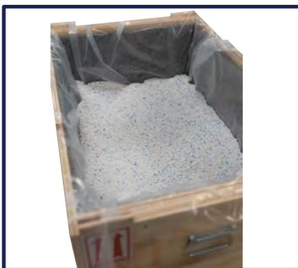
Pour CellBlock EX into crate liner, covering liner by a minimum of 1/2". Place battery in crate, covering with a minimum of 1/2" CellBlock EX on all sides.
