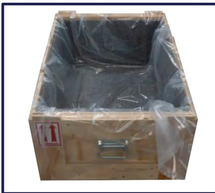
Remove top or appropriate side for proper loading of module/pack. Place liner inside the unit.
